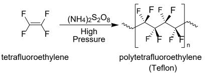
Tetrafluoroethylene is virtually resistant to all chemicals and forms a surface which is non-stick. Tetrafluoroethylene also maintains these properties over a temperature range of -270 to 385 Celsius.
